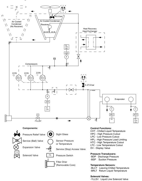
Low pressure liquid refrigerant enters the evaporator and is evaporated and superheated by the heat energy absorbed from the chilled liquid. Low pressure vapour enters the compressor where pressure and superheat are increased. The high pressure vapour is fed to the air cooled condenser coil and fans where heat is removed. The fully condensed and subcooled liquid passes through the expansion valve where pressure is reduced and further cooling takes place before returning to the evaporator.
